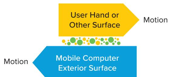
Figure 1: Three-Body Abrasion
